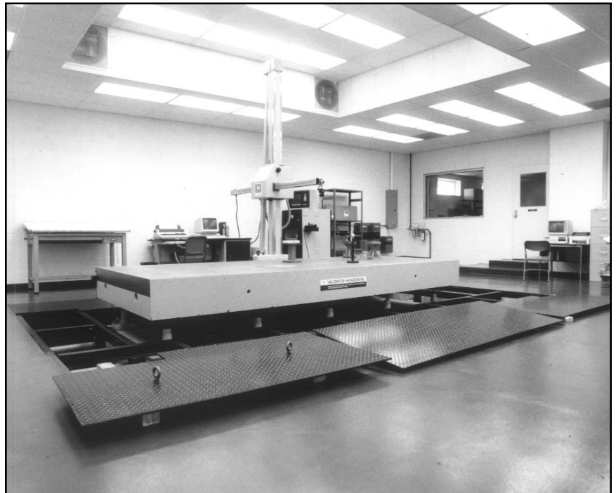
Single Arm CMM on Air Support Inertia Base with Removable Isolator Access Plates
