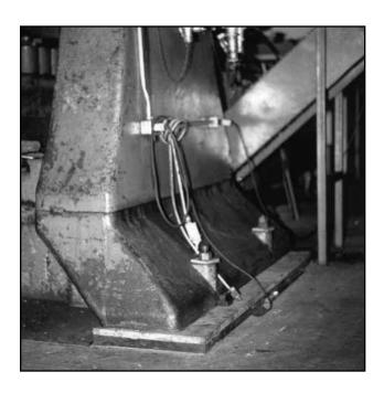
structure, exceeding the Canadian code by 80%! It was felt that the excessive transmission was because the 6-year-old neoprene pads had age-hardened and stiffened with time, rendering them useless as vibration and shock isolators.
